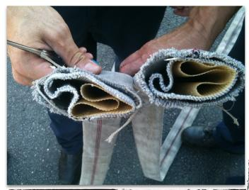
Delamination can occur at any part of the hose line and not just the ends. If the hose feels "lumpy" in any part than it is suspect. This is a hose line that was cut at the middle of a 50' section. It is clear that the liner has separated from the exterior jacket. When water pushes through the hose it will create turbulence that can cause the liner to twist and occlude your fire flow.
