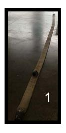
To create the Engineer roll, fold the 50' section of 3" in half pulling the male coupling back approximately 3' from the female, then begin rolling from the fold until the entire section is rolled tight
