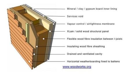
At The insulation is usually placed on the outside of the CLT panel to reduce expansion and contraction issues and to make available for use as much of the floor space inside the building as possible.
