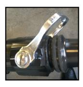
Check the bale, make sure it is free of cracks and is tight to the nozzle, ensure that it operates the interior valve by opening and closing the bale and looking to see that the valve actuates
