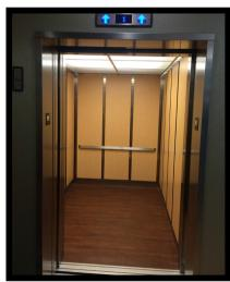
To take control of the elevator insert the key into the fire service slot and turn to "ON" this will return all cars on the system to the main level or level of the fire control panel
